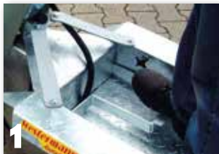
1: easy lifting up of scraper via foot rotor lift
